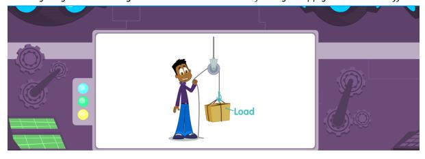
A pulley is made from a wheel with a groove around its circumference. The wheel rotates around an axle and a piece of rope or string is fed through the groove.
