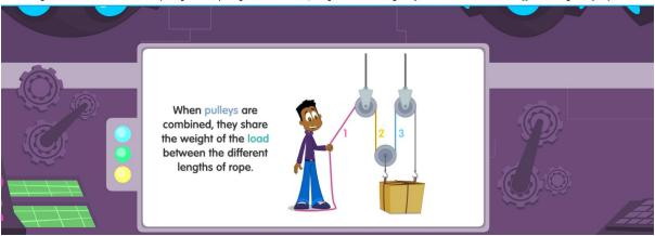
Pulleys are made by looping a rope over one or more wheels. They are often used to lift heavy objects: pulling down on one end of the rope creates an upward pull at the other end. Looping the rope over more wheels increases the upward force. Using two wheels means you can lift something twice as heavy using the same force.
